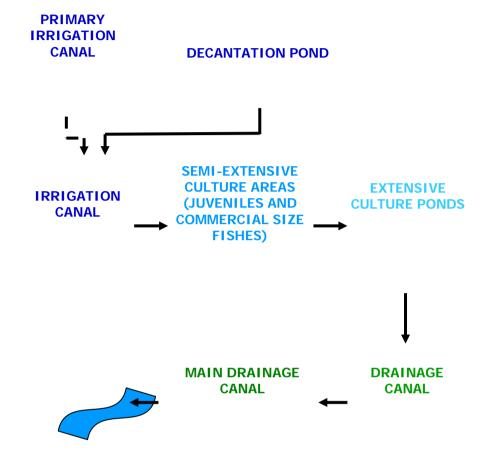
Figure 4. Water control scheme at *Veta la Palma* aquaculture operation.
